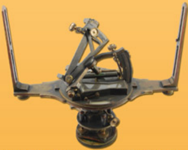
A "Burt's" solar compass used for surveying, ca. 1880.
