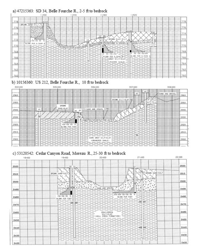
Figure 10. Stratigraphic cross sections of valley alluvium from three West River bridges. Source: SD DOT design plans.
