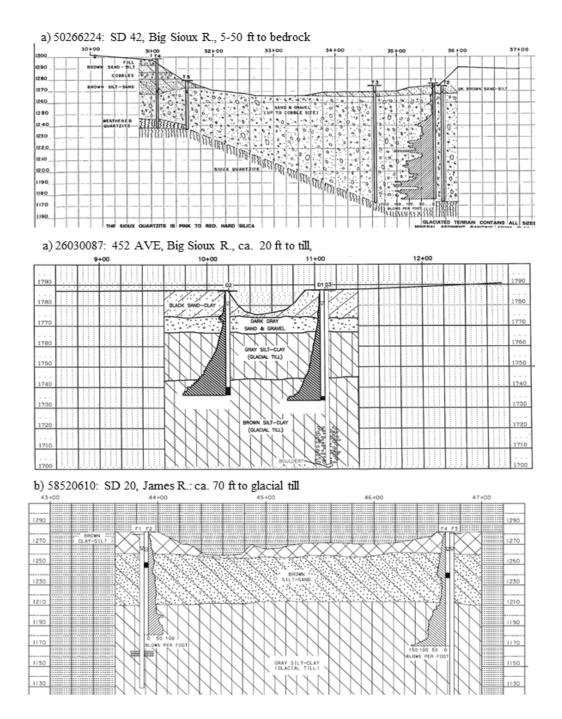
Figure 9. Representative stratigraphic cross sections of alluvium at three East River bridges (source SD DOT design plans.
