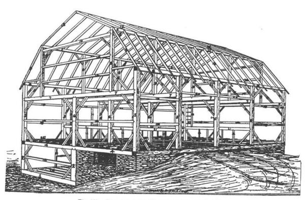
Fig. 120. General Framing Plan for a Heavy Timber Barn.
