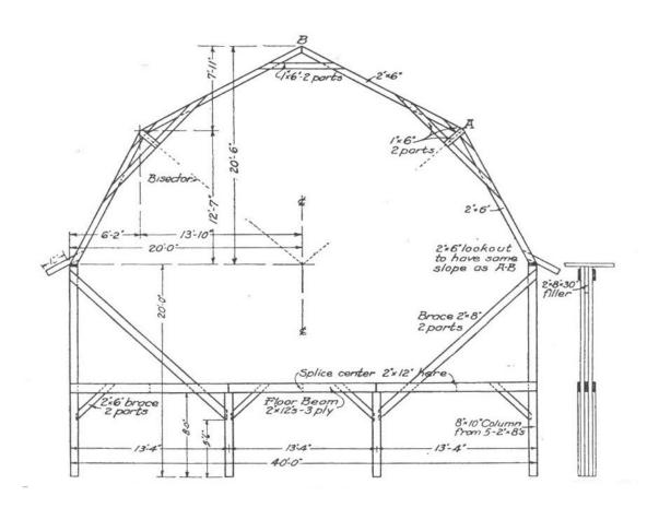
Wing Joist Frame (Plank Frame) Bent
