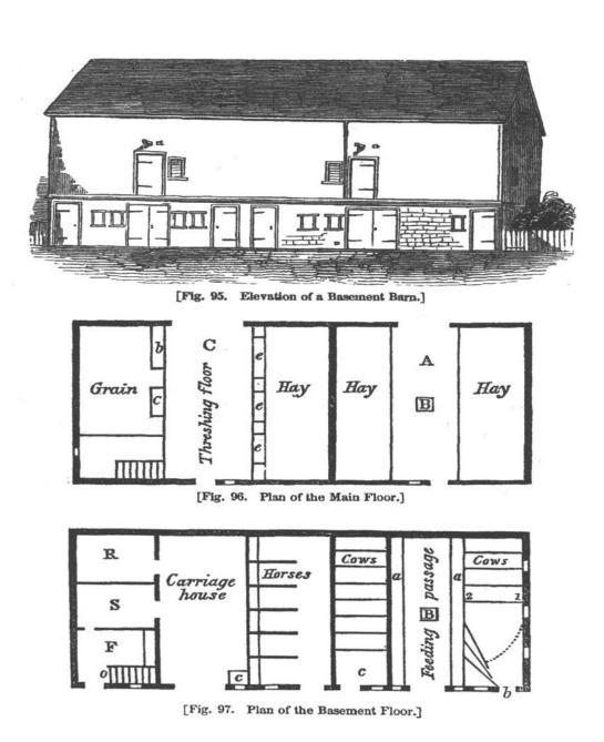
Elevation and plans of a "basement barn" for A. J. Downing, *The Architecture of Country Houses* (1852).
