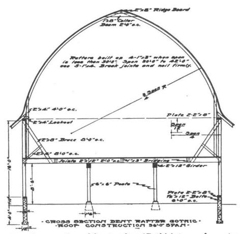
FIG. 80.—Cross-section of bent rafter (Gothic) type of construction.
