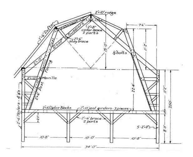
Shawver Truss (Plank Frame) Bent
