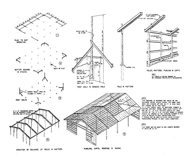
Plans for a pole barn (post frame construction), adapted from the U.S.D.A. Midwest Plan Service plan number 5780.
