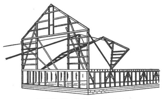
Fig. 134. How the Bents are Raised.
