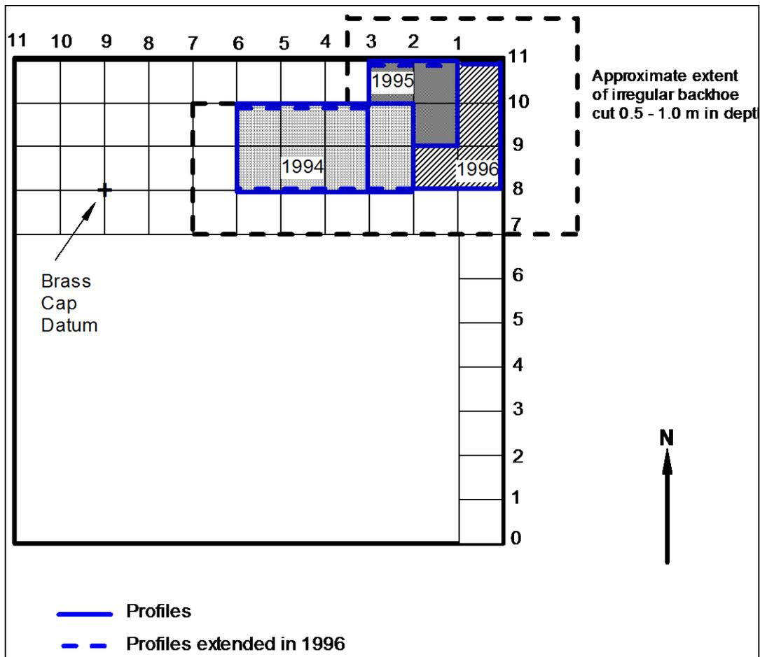
Figure 78. Plan view of the Area B excavation grid identifying the 1995 brass cap datum position and the location of the four new units opened in relation to those excavated during the 1994 and 1995 seasons.
