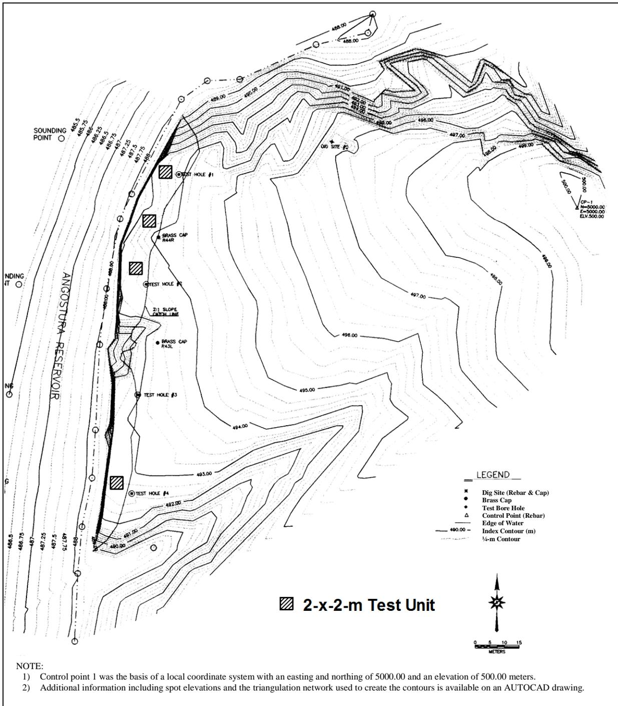
Figure 114. Contour map prepared for the 1999 stabilization plan proposed for the Ray Long site (39FA65). Brass cap datums, 2-x-2-m test units, and geotechnical test bore holes indicated.
