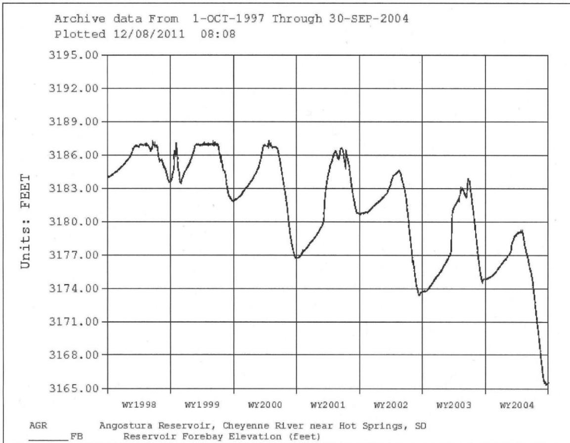
Figure 107. Reclamation Hydromet plot for water elevations at Angostura Reservoir from water-years 1998 to 2004.
