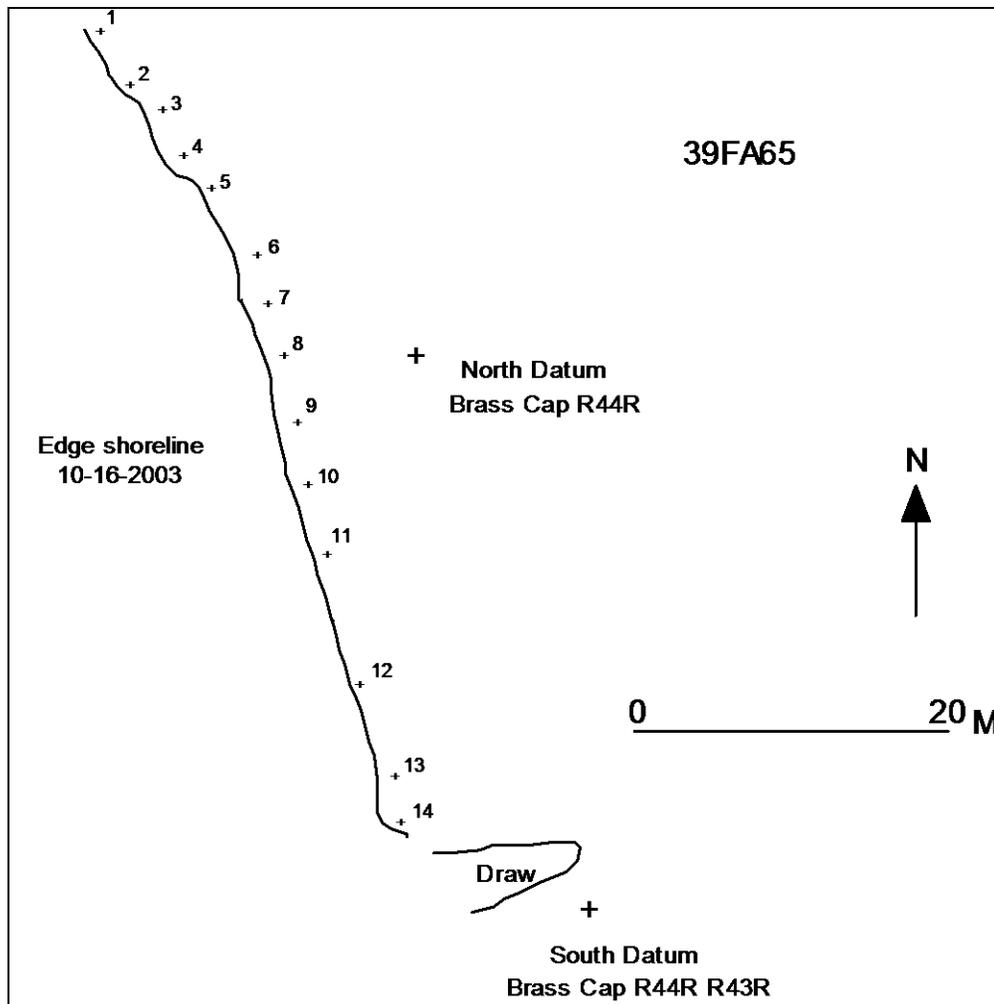
Figure 128. The edge of the shoreline (cut bank) on October 16, 2003. Points 1-14 were measured (taped) from the north and south datums (see Tables 17 and 18, below).
