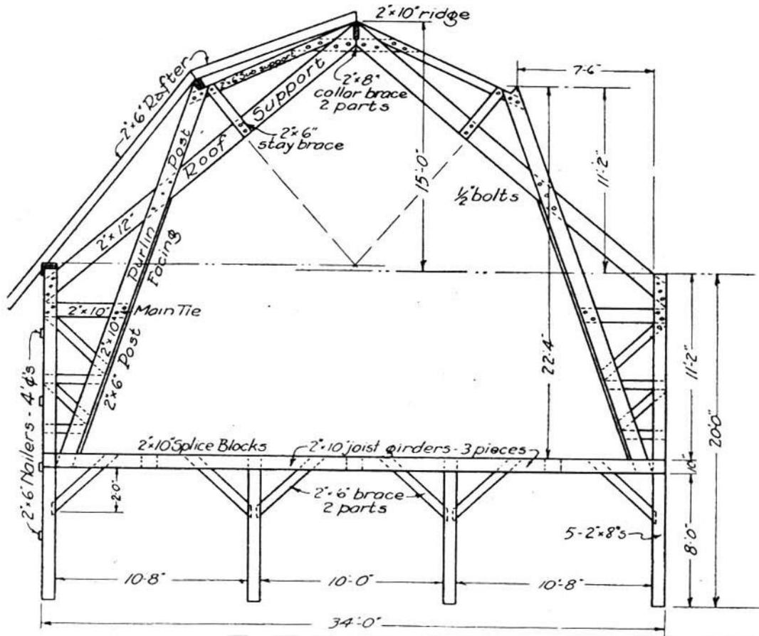
Shawver Truss (Plank Frame) Bent
