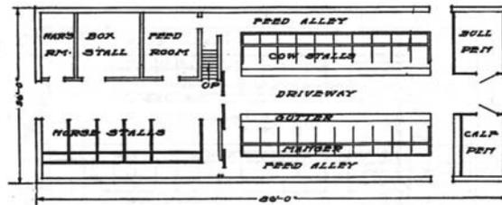
Fig. 34.—Floor plan of a typical general farm barn.
