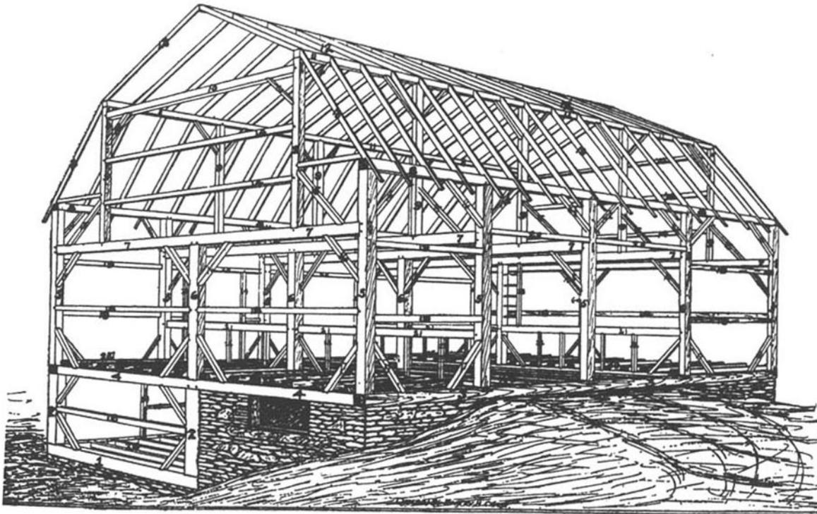
Fig. 120. General Framing Plan for a Heavy Timber Barn.
