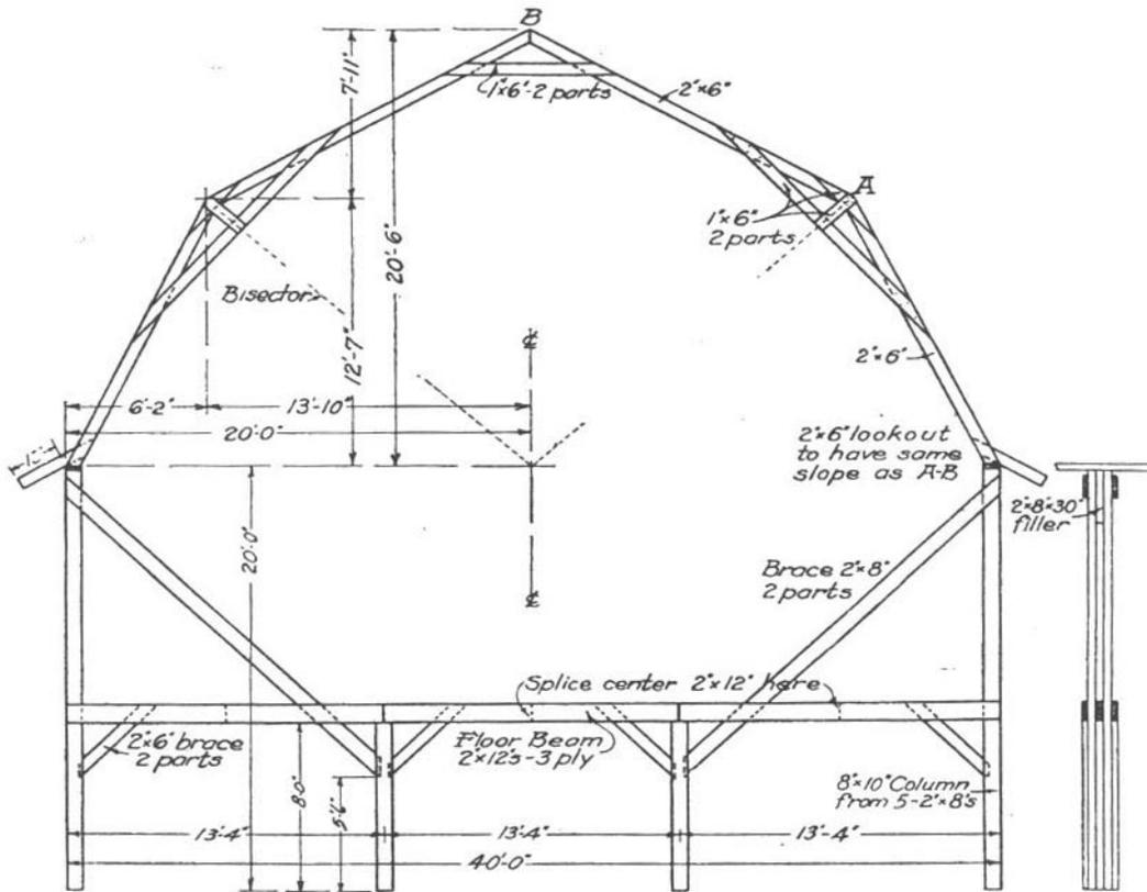
Wing Joist Frame (Plank Frame) Bent
