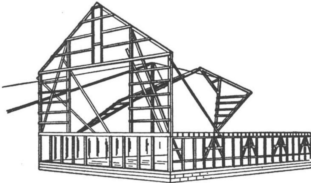
**Fig. 134. How the Bents are Raised.**
