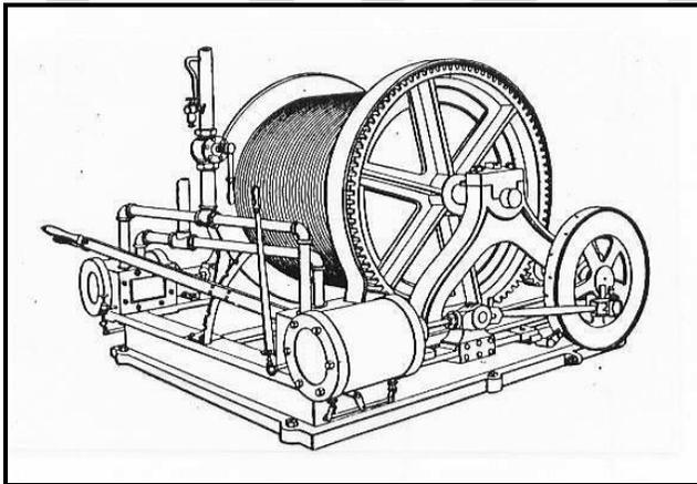
Figure 3.19: Single-drum geared steam hoists were the most common power type between the 1870s and 1910s. Gasoline and electric models became popular afterward. Source: International Text Book Company, 1906, A50:8.
