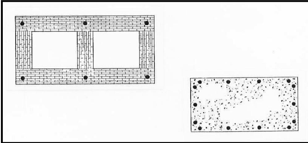
Figure 3.49: The plan views depict foundations for geared double-drum steam hoists. The foundation at left features wells for the hoist's cable drums. Source: Twitty, 2002:242.
