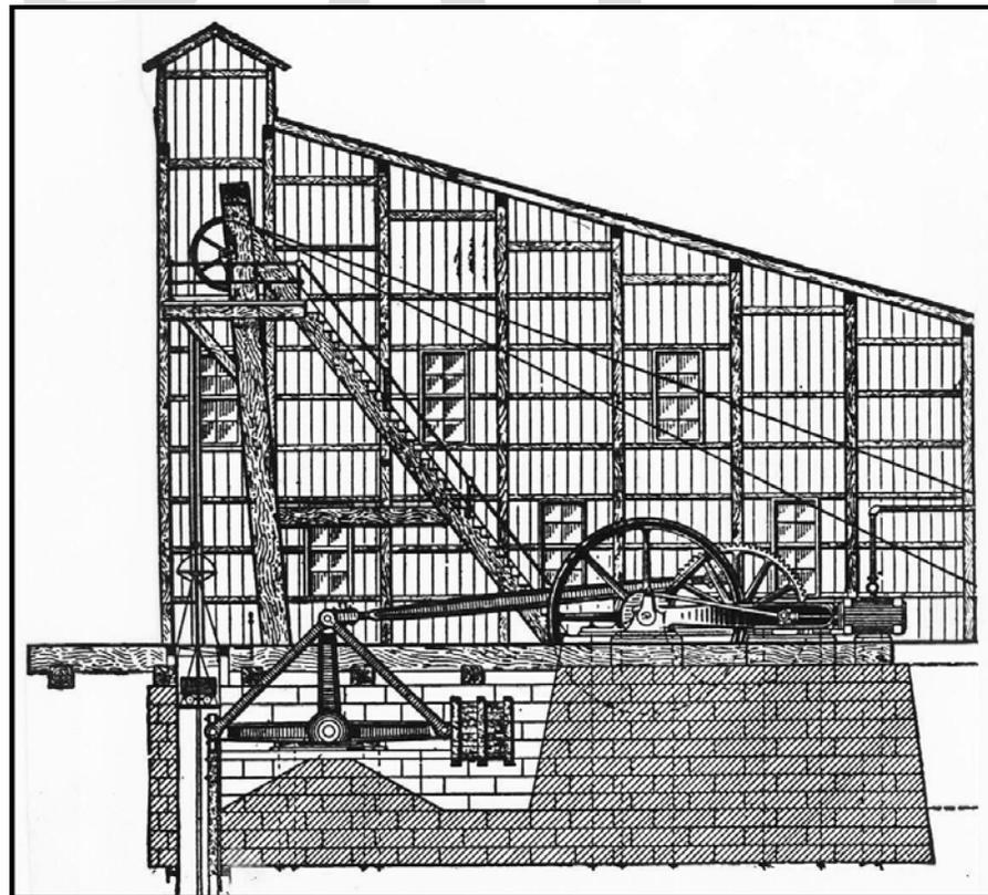
Figure 3.32: Shaft houses enclosed the shaft collar, headframe, hoist, power system, and usually the blacksmith shop. The shaft house in the profile also features a Cornish pump and steam engine. Source: International Textbook Company, 1899, A43:3.
