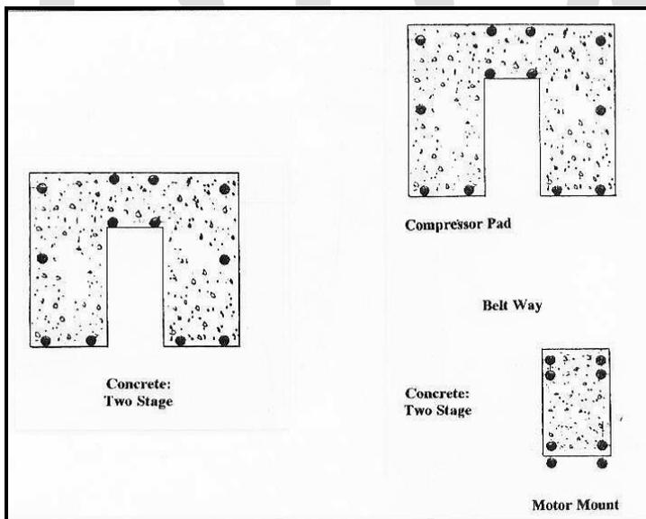
Figure 3.41: Compact duplex compressors were mounted to foundations like those in the above plan view. The foundation at left anchored a steam-powered unit, and the one at right was for a belted version, which became popular by the 1910s. Source: Twitty, 2002:109.
