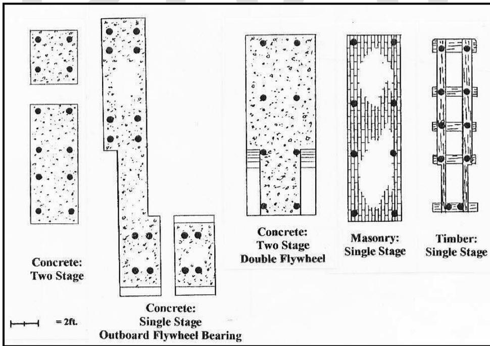
Figure 3.37: The plan view depicts foundations for straight-line compressors. Source: Twitty, 2002:145.
