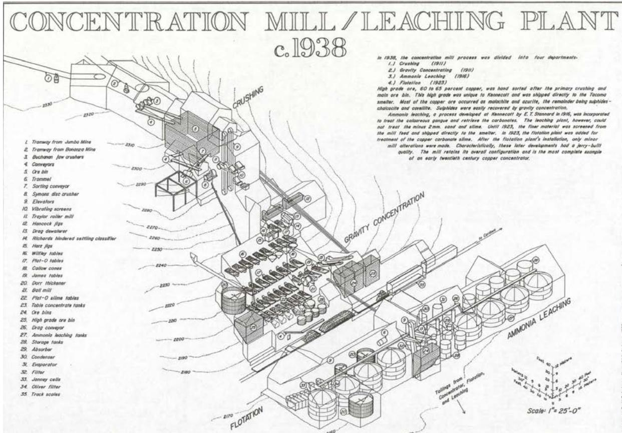
Figure 3.60: Concentration Mill/Leaching Plant diagram.
