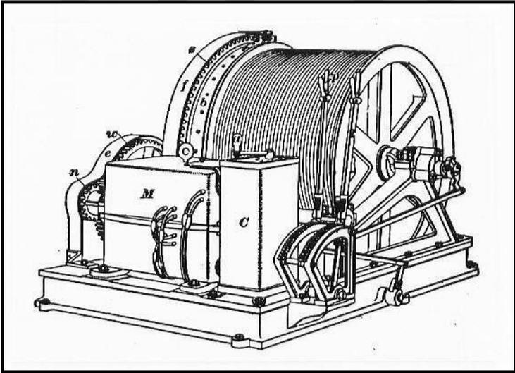
Figure 3.22: The single-drum electric hoist grew in popularity during the 1910s where power was available. The motor is in the case in front, drive gearing is at left, and the upright box is a speed controller. Source: Twitty, 2002:224.
