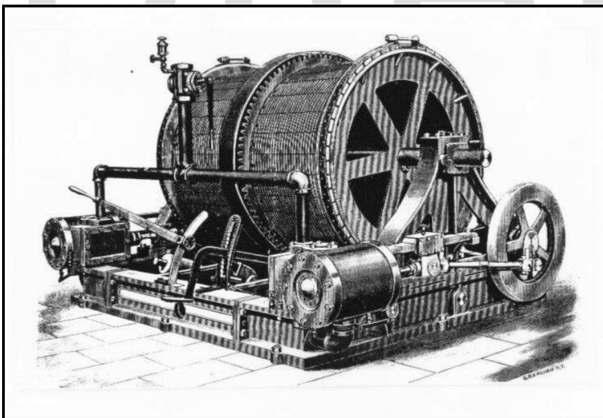
Figure 3.48: Rear quarter view of a geared double-drum steam hoist. Double-drum hoists, hallmarks of significant ore production, achieved balanced hoisting with two vehicles. Source: Ingersoll Rock Drill Company, 1887:65.
