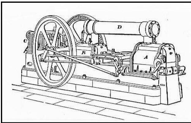
Figure 3.36: The line drawing depicts a straight-line steam compressor that provided two stages of compression. One compression cylinder is at right, another is at center, and the steam drive cylinder is at left. The flywheels imparted momentum to the machine. Source: International Textbook Company, 1899, A20:32.
