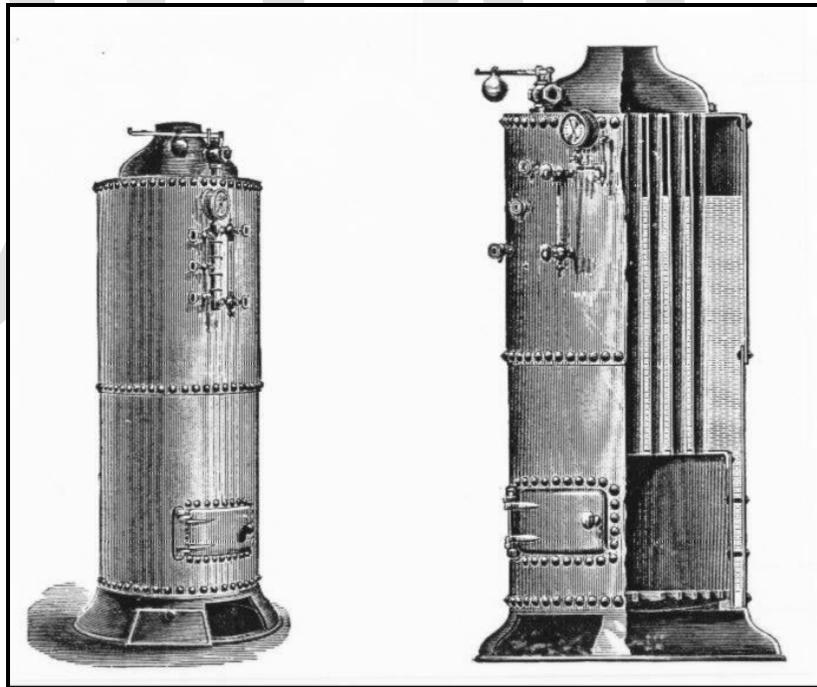
Figure 3.14: Upright boilers were the least expensive and most portable type of boiler, but also inefficient. Flue gases rose from the firebox at bottom, through the flue tubes, and out a smokestack at top. Note the water level sight tube, pressure gauge, and pressure valve. Source: Rand Drill Company, 1886:47.
