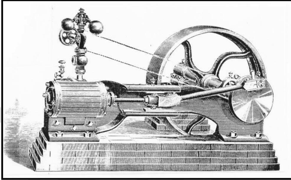
Figure 3.93: Until electricity became available during the 1910s, horizontal steam engines powered nearly all concentration mills. A drive belt passed around the flywheel to a mill's system of driveshafts. Note the masonry foundation. Source: Ingersoll Rockdrill Company, 1887:53.
