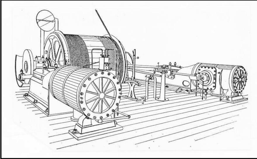
Figure 3.51: Rear quarter view of a direct-drive single-drum steam hoist. Powerful steam cylinders flank the hoist's controls, and the drive-rods are directly coupled to the cable drum. Source: International Text Book Company, 1906, A50:16.
