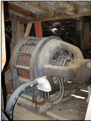
Figure 3.94: By the 1910s, mining companies increasingly used electric motors to power their mills, provided electricity was available. Source: Carol Beam, Boulder County Parks and Open Space, Colorado.
