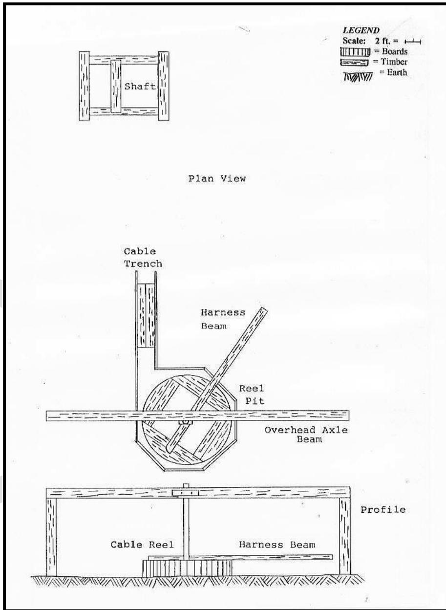
Figure 3.13: The plan view, top, and elevation, bottom, depict a horizontal reel horse whim, which was a universal prospecting hoist prior to the 1880s. The reel was mounted to an axle on a timber footer buried in the floor of a plank-lined pit. Usually, only the pit and cable trench remain at prospect shaft sites today. Source: Twitty: 2002:158.
