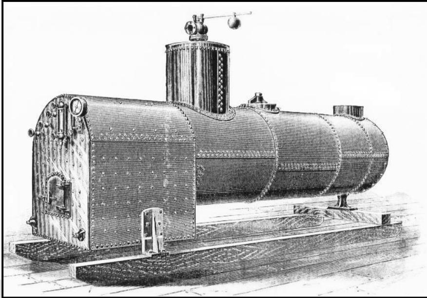
Figure 3.15: The locomotive boiler was one of the most popular steam generators. Flue gases traveled from the firebox at left through flue tubes in the tank and out a smokestack at right. Source: Rand Drill Company, 1886:45.
