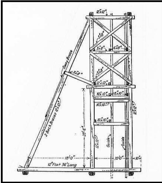
Figure 3.45: The headframe at left is a four-post derrick type. Production-class headframes such as the one illustrated tend to be higher than 25 feet. Source: *Engineering & Mining Journal* 12/28/17 p1216.
