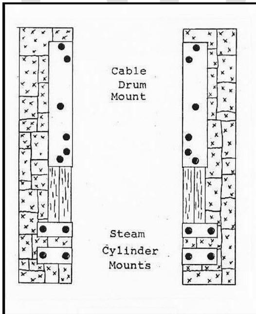
Figure 3.52: The plan view depicts a typical foundation for a direct-drive single-drum steam hoist. Such foundations are usually less than 14 by 17 feet in area. Source: Twitty, 2002:241.
