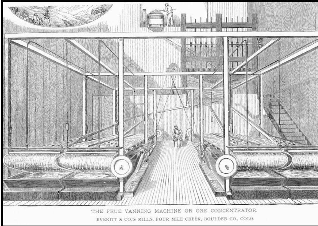
Figure 3.90: The Everett Mill, which operated in Colorado during the late 1870s, employed several Frue vanners to concentrate gold ore. As the vanner vibrated, finely ground ore settled against the broad rubber belt while water jets and a scraper removed light waste material. Note the stamp battery at upper right. Source: *Engineering & Mining Journal* 11/24/77, p387.
