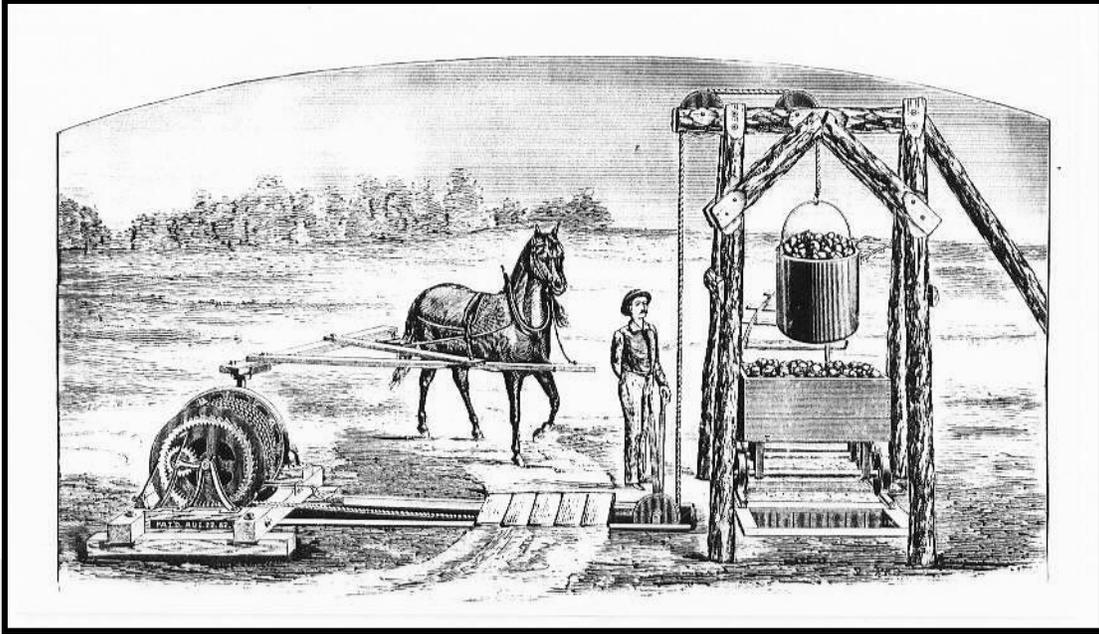
Figure 3.12: Horse whims were the most primitive type of mechanical hoist, and because of their simplicity and portability, they were a favorite among prospectors. The unit shown is a geared whim, which was popular from the 1880s through the 1910s. The hoist operator controlled a brake and clutch via levers mounted to the shaft collar. The control linkages and hoist cable passed through the trench. Source: Ingersoll Rock Drill Company, 1887:60.
