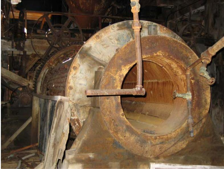
Figure 3.83: Rod mills became popular for fine grinding by the 1910s. As the entire cylinder slowly rotated, tumbling steel rods in the chamber ground screened ore into a slurry. A hatch covered the opening. Source: Carol Beam, Boulder County Parks and Open Space, Boulder, Colorado.
