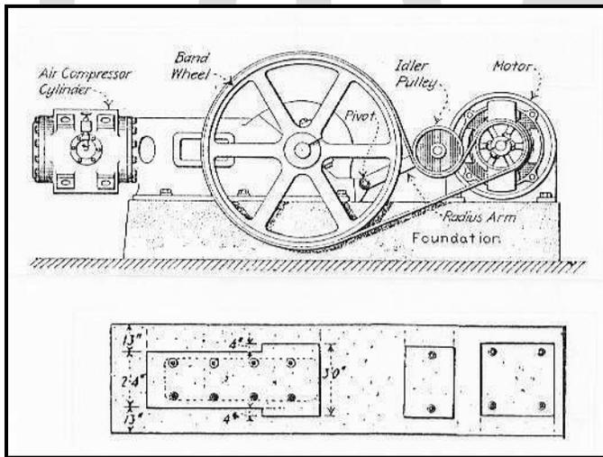
Figure 3.44: The profile illustrates the type of small, belted compressor popular between the 1910s and 1940s. The plan view shows the foundation, which features mounts for the compressor and motor. Source: Eric Twitty.
