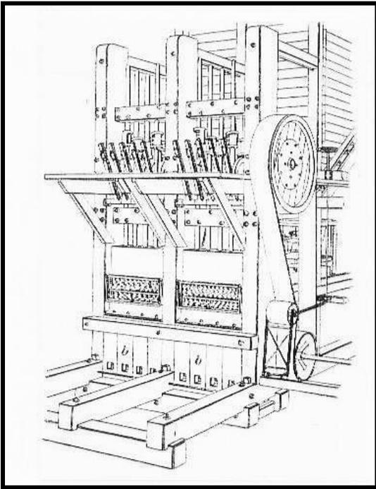
Figure 3.79: The quarterview illustrates the front of a stamp battery, which provided secondary crushing at some mills. Stamp rods are visible between the timber posts, and their heavy iron shoes pounded ore in the battery boxes below. The battery boxes are bolted to pedestals of upright timbers, which are often the only remnants of stamp batteries today. Source: International Textbook Company, 1899, A43:27.
