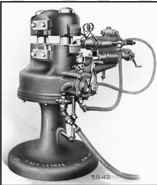
Figure 3.58: Shortly after 1910, leading rockdrill makers introduced a compact drill-steel sharpening machine around 5 feet high. The device, purchased by well-capitalized mining companies, expedited the drill-steel sharpening process. Source: *Ingersoll-Rand*, 1913:2.
