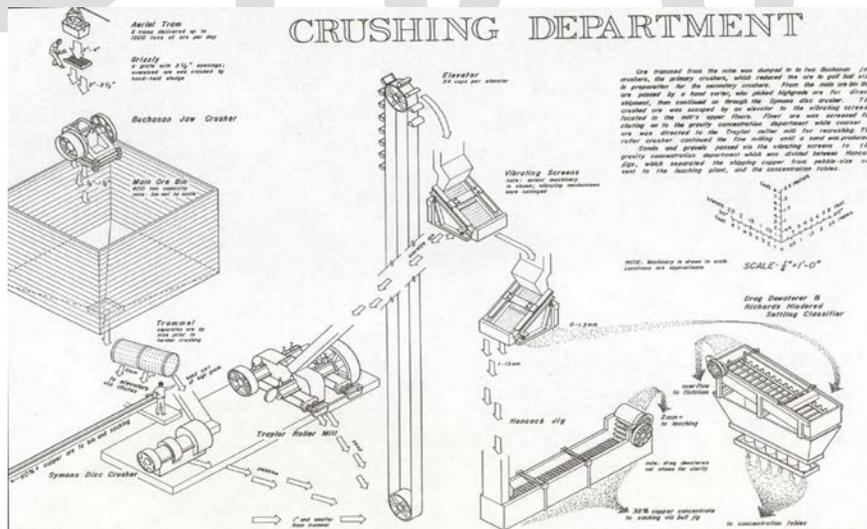
Figure 3.62: Crushing diagram.
