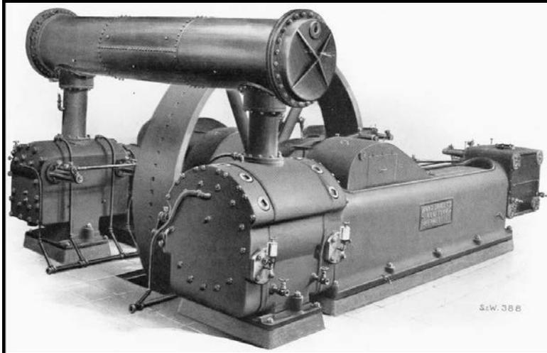
Figure 3.40: During the 1890s, the above form of duplex compressor became popular. Originally, these machines were powered by steam, and by the 1900s, some were also belted to motors where electricity was available. Source: Rand Drill Company, 1904:12.
