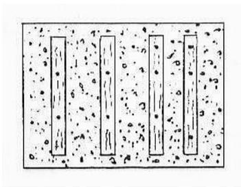
Figure 3.42: The illustration at left is a plan view for a V-cylinder compressor foundation (see Figure 3.35). Timber footers are embedded in a concrete rectangle around 3 by 4 feet in area. Source: Eric Twitty.
