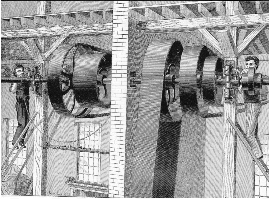
Figure 3.95: A system of overhead driveshafts and belts was the most common means of transferring motion from a mill's engine to its various appliances. Source: *Mining & Scientific Press* 9/1/83, p129.
