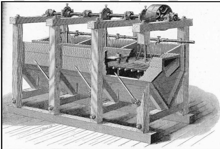
Figure 3.89: The jig was an effective concentration device popular from the 1860s through the 1910s. The crank at top moved three screen plungers up and down in the water-filled cells, illustrated by the cut-away view. The agitating action classified crushed ore particles by size or weight, depending on the application. Source: *Mining & Scientific Press* 8/9/90, p83.
