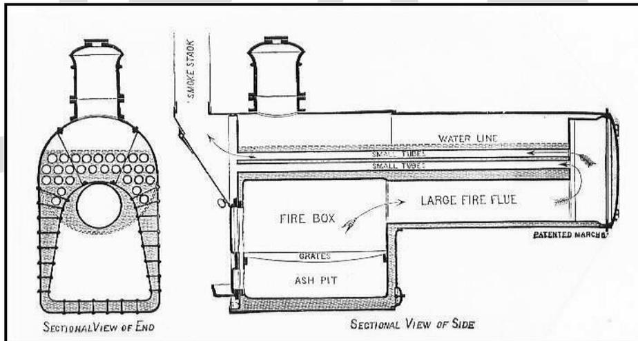
Figure 3.16: The Pennsylvania boiler was portable, stood on skids, and provided greater fuel economy than the locomotive type. Note the path traveled by the flue gases, which prolonged contact with the boiler surfaces. Source: Rand Drill Company, 1886:46.
