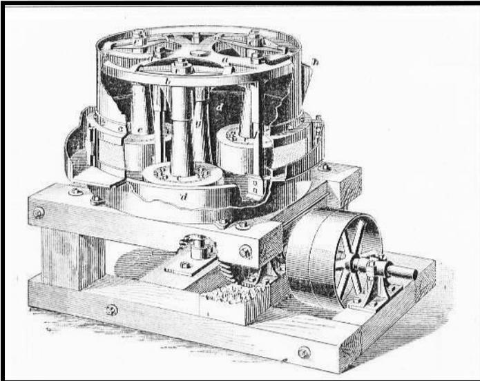
Figure 3.82: The device known as the Huntington mill saw two applications. At concentration facilities, it provided secondary and tertiary crushing, and at amalgamation mills, the device simultaneously ground and amalgamated gold and silver ores. The driveshaft at right turned a capstan in the mill's pan, which caused the rollers to grind screened ore against the pan's cast iron walls. Note the foundation. Source: International Textbook Company, 1899, Z43:47.
