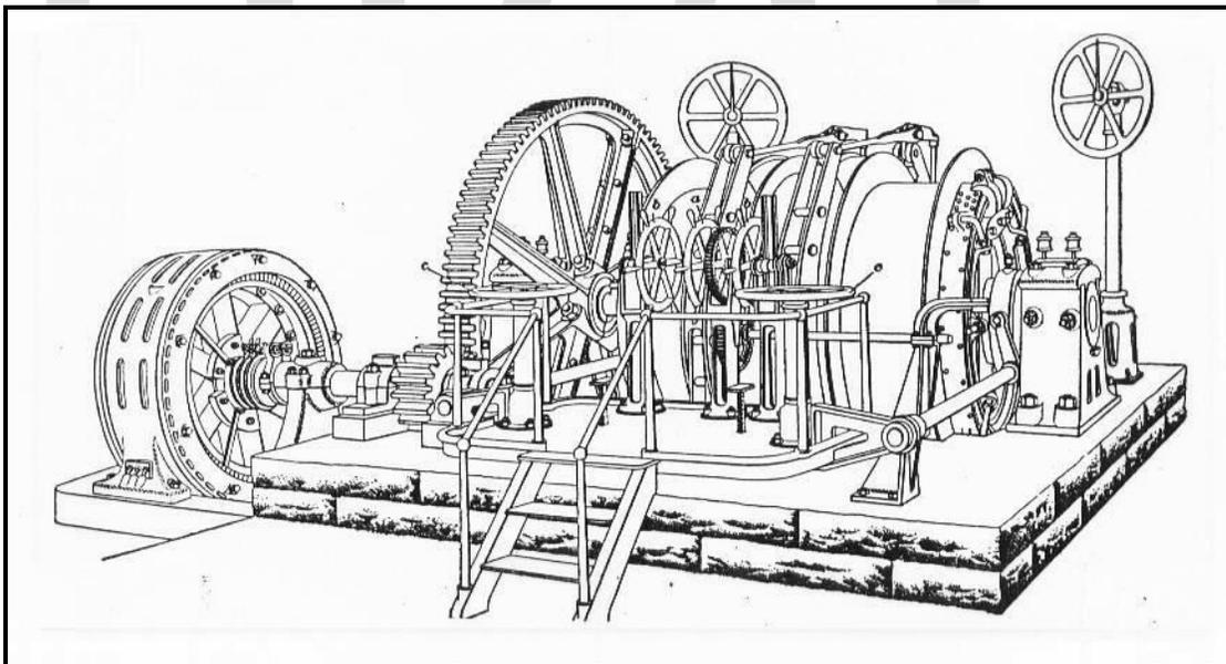
Figure 3.50: Rear quarter view of a double-drum electric hoist. The motor at left drove the dual cable drums via the large bull gear. Such hoists facilitated heavy production, saw use after the 1910s, and were popular among well-capitalized companies by the 1930s. Note the foundation. Source: International Textbook Company, 1906, A50:40.
