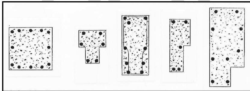
Figure 3.25: Hoist foundation plan views. Single-drum steam hoists were bolted to foundations like the one at left, and the other foundations were for various types of gasoline hoists. Source: Twitty, 2002:187, 241.
