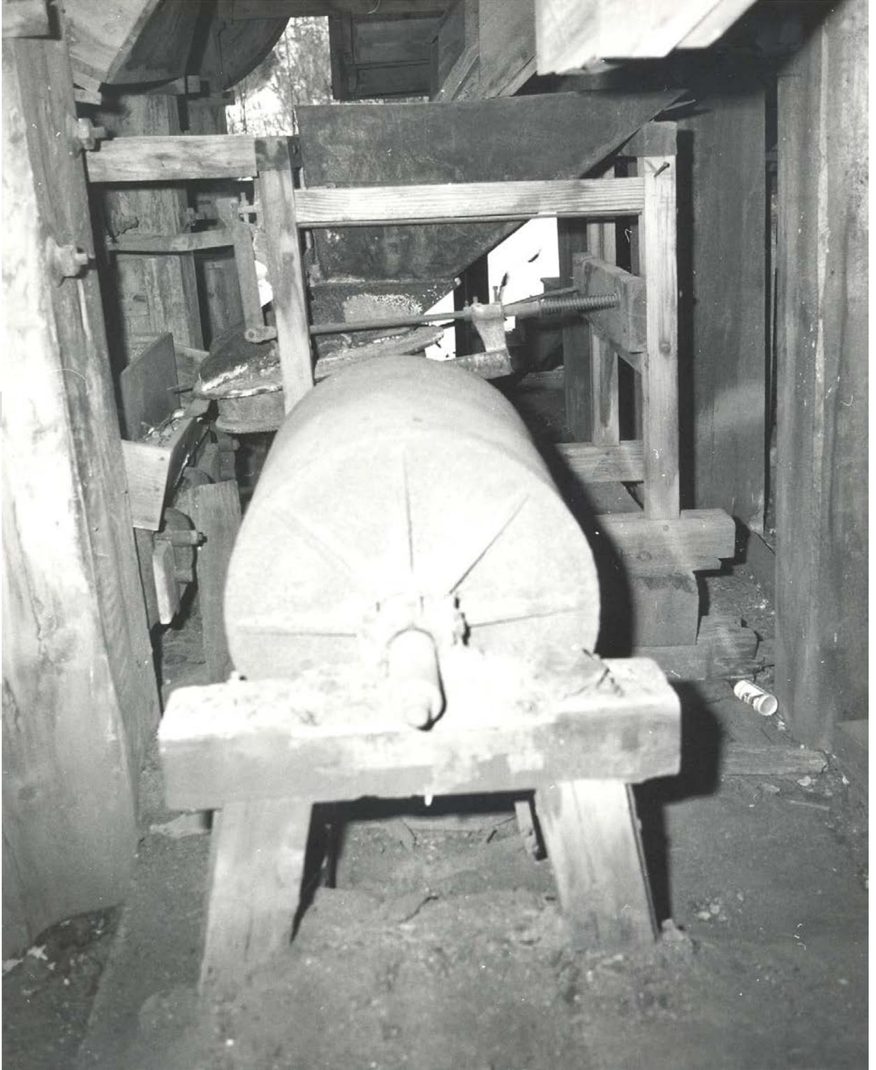
Figure 3.85: Ball Mill from the Standby Mine near Rochford. Courtesy South Dakota State Historical Society.
