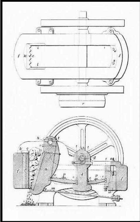
Figure 3.77: The plan view, top, and profile, bottom, illustrate a jaw crusher, which provided initial crushing at most mills. Source: International Textbook Company, 1899, A43:2.
