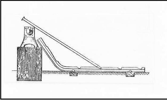
Figure 3.57: The profile illustrates a backing block, the steel bar on the floor that shop workers used to brace hot drill-steels during sharpening. The drill-steel rests in a divot in the bar, and its neck rests against an anvil on a timber stand. Backing blocks were embedded in the shop floor adjacent to the forge. Source: *Engineering & Mining Journal*, 1916:14.
