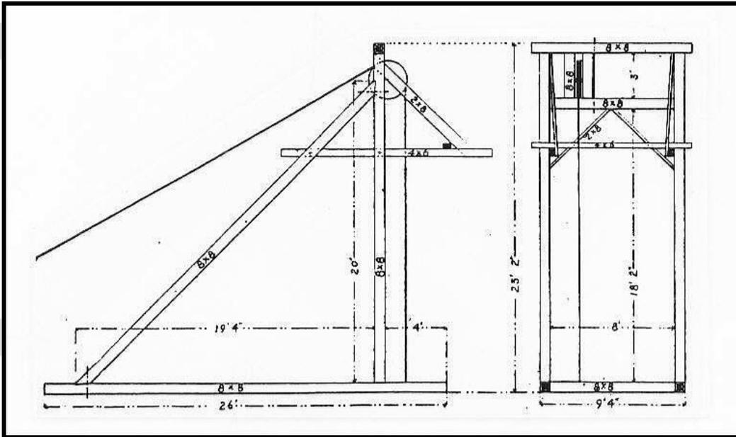
Figure 3.18: The two-post gallows headframe was the most common type for prospect shafts. Sinking-class versions tended to be less than 25 feet high and stood on timber footers. Source: *Engineering & Mining Journal* 3/7/03 p366.
