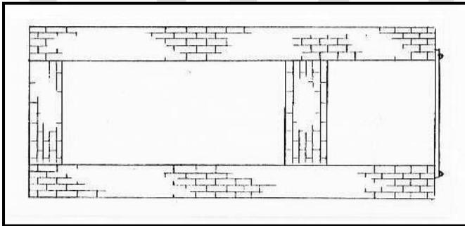
Figure 3.54: Few return-tube boilers currently remain intact and have been reduced to setting remnants and foundations, such as the one in the plan view. Source: Twitty, 2002:145.
