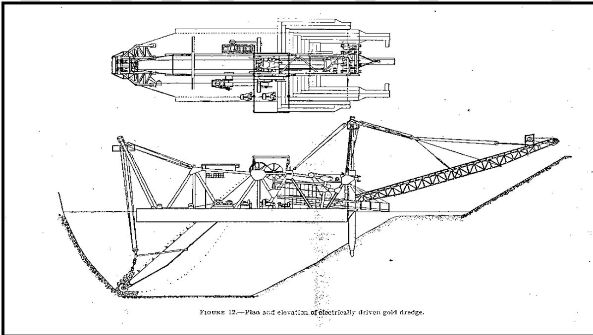
FIGURE 12.—Plan and elevation of electrically driven gold dredge.
