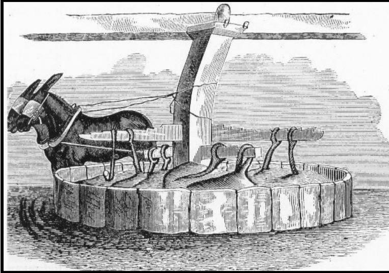
Figure 3.71: The ages-old arrastra was the most primitive ore treatment facility in the Rocky Mountain west. The operator shoveled gold ore into the interior, added mercury, and waited for the rotating muller stones to grind the material into sand and slurry. As the ore fractured, mercury amalgamated with the gold. Because arrastras were simple and inexpensive, they were used by prospectors on the frontier. Source: *Mining & Scientific Press* 5/26/83.
