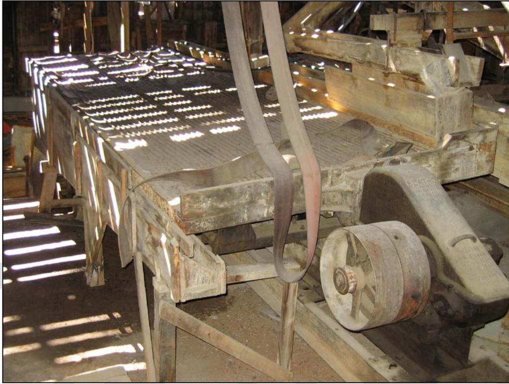
Figure 3.92: Following its introduction around 1898, the vibrating table was one of the most popular and effective concentration appliances throughout the Rocky Mountain west. An eccentric cam under the guard at right imparted a vibrating motion to the tabletop, and the vigorous action caused heavy metalliferous material to settle against the riffles. Water currents washed the light waste off. Source: Carol Beam, Boulder County Parks and Open Space.
