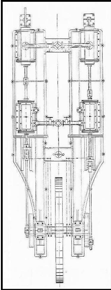
Figure 3.38: The plan view shows a typical pre-1910 duplex steam compressor. The compression cylinders are at top, the steam drive cylinders are at center, and the flywheel is at bottom. Source: Ingersoll Rock Drill Company, 1887:34.
