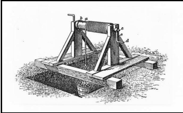
Figure 3.11: The windlass was an institution among prospectors, and nearly all shafts less than 100 feet deep were equipped with this simple, inexpensive, and portable type of hoist. Source: Twitty, 2002:145.
