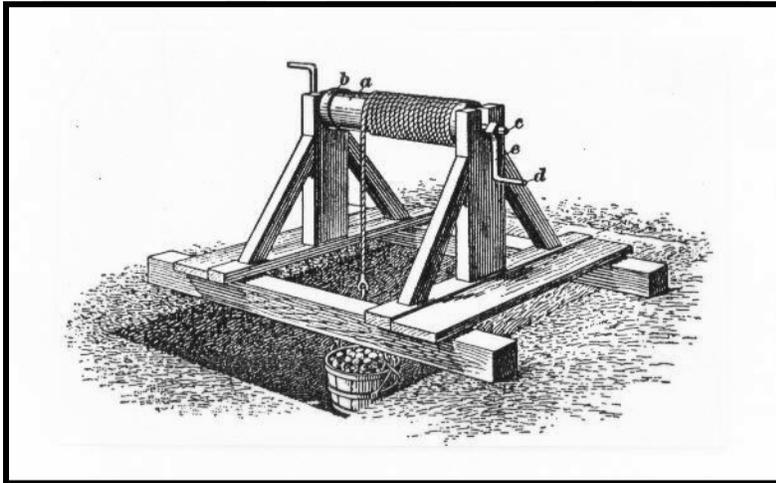
Figure 3.11: The windlass was an institution among prospectors, and nearly all shafts less than 100 feet deep were equipped with this simple, inexpensive, and portable type of hoist. Source: Twitty, 2002:145.
