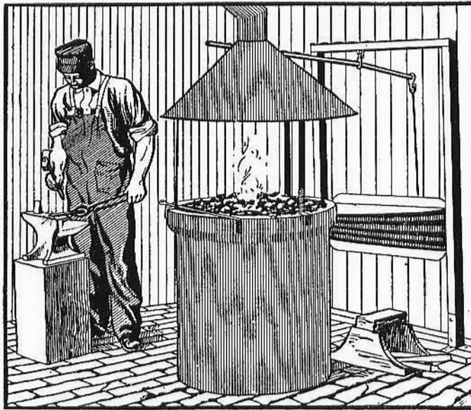
Figure 3.26: The illustrated shop is representative of those at prospects and small mines. Such shops usually consisted of little more than a forge, an anvil, and hand-tools, which restricted work to drill-steel sharpening and the manufacture of light hardware. Source: Drew, 1910:1.
