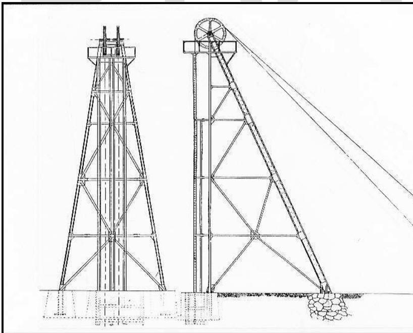
Figure 3.46: The illustrated headframe is a production-class two-post gallow's structure known as a Montana type. These headframes were usually tall, well-built, and stood over deep shafts. Source: Twitty, 2002:233.
