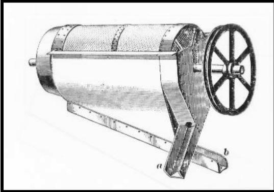
Figure 3.81: Most mills relied on trommel screens to sort crushed rock between processing stages. Source: International Textbook Company, 1899, A43:12.
