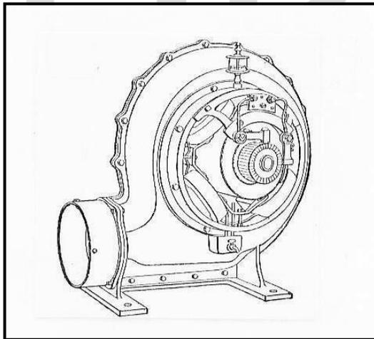
Figure 3.34: At left is a common ventilation blower used to force fresh air underground. Ducting was fastened to the nozzle, and a belt turned the machine. Source: International Text Book Company, 1899, A41:146.
