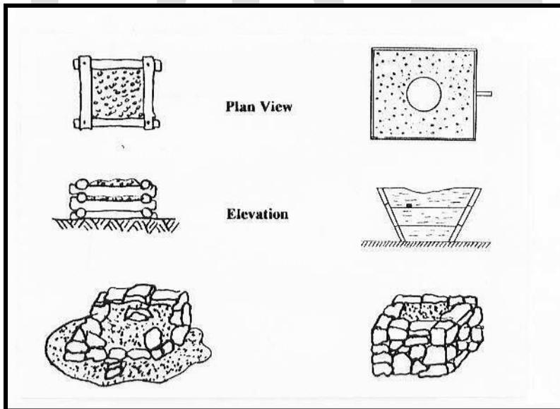
Figure 3.27: Above are examples of the common forges used in blacksmith shops. At upper left is a gravel-filled log forge, at right is a wood box forge, and at lower right is a dry-laid rock forge. Over time, rock forges decay and collapse, and manifest as the remnant at lower left. Source: Eric Twitty.
